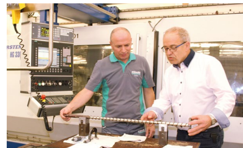
Rotating parts, such as screws, are also manufactured at Arburg with a fully synthetic cooling lubricant from the Colometa family. Siegfried Finkbeiner, Head of Production (right), is responsible for the production processes.
